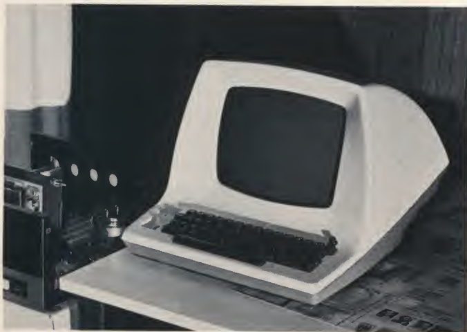
The clean lines of the ADM-3A, shown being used with an SWTP M6800 system. An 80-character line is greatly appreciated after using terminals with a 32- or 64-character line width.
